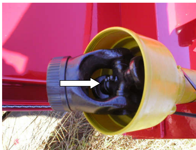
Lubricating Driveshaft Slip Joints
