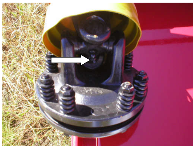
Lubricating Universal Joints
